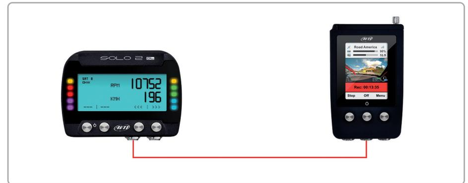
To connect Solo 2 DL to LCU-One CAN connect 5 pins Binder connector placed bottom left of Solo 2 DL to 5 pins Binder connector of LCU-One as shown here below.
