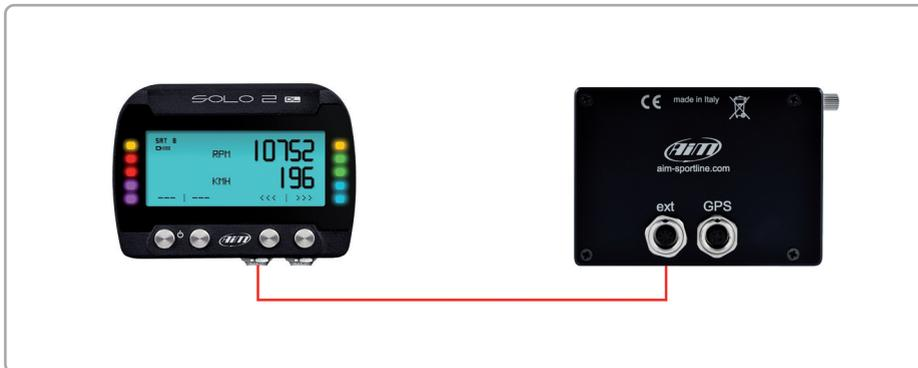
To connect Solo 2 DL to SmartyCam GP HD use SmartyCam CAN cable and connect 5 pins Binder connector placed bottom left of Solo 2 DL to 7 pins central Binder connector of SmartyCam HD as shown here below.
